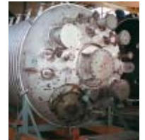
Figure 1: Container made of highly corrosion resistant duplex stainless steel
