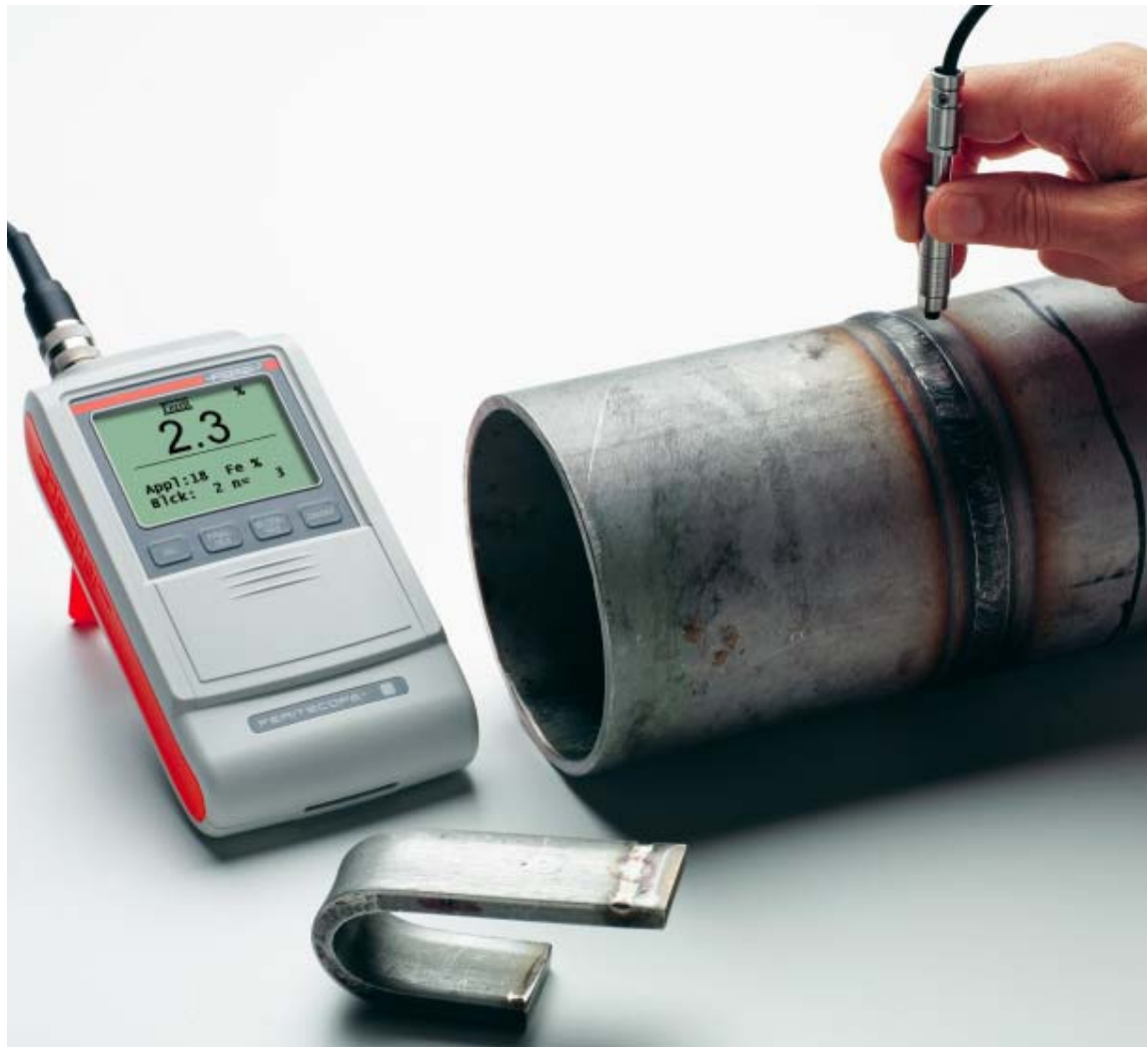
Determination of the ferrite content in the area of weld seams using the FERITSCOPE® FMP30
