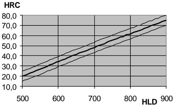
**Fig. 4:** Conversion of Hardness Leeb, HL, into HRC as a typical example for conversion tables stored in rebound hardness testers. These curves are experimentally generated by material samples of different hardness measured by rebound and Rockwell test.
