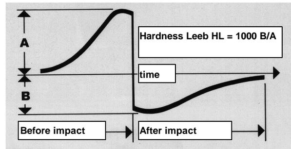
Fig. 3: Voltage signal generated by the impact body penetrating through the coil. The signal is shown before and after the impact
