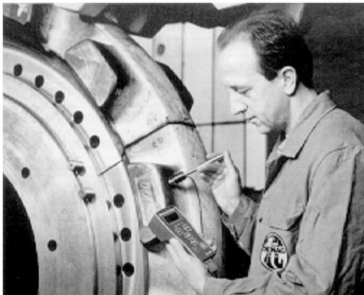
Fig. 1: Typical Rebound hardness testing application
