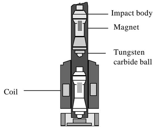
Fig. 2: Cross-cut of a typical impact device
